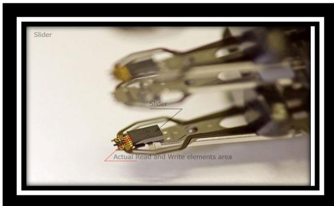
The slider is aerodynamically constructed to create an air bearing for the read heads.
