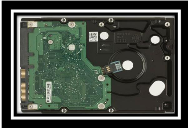
The green component shown above is called the Printed Circuit Board or PCB. The PCB holds the controlling electronics. The black case is called the Hard Disk Assembly.
