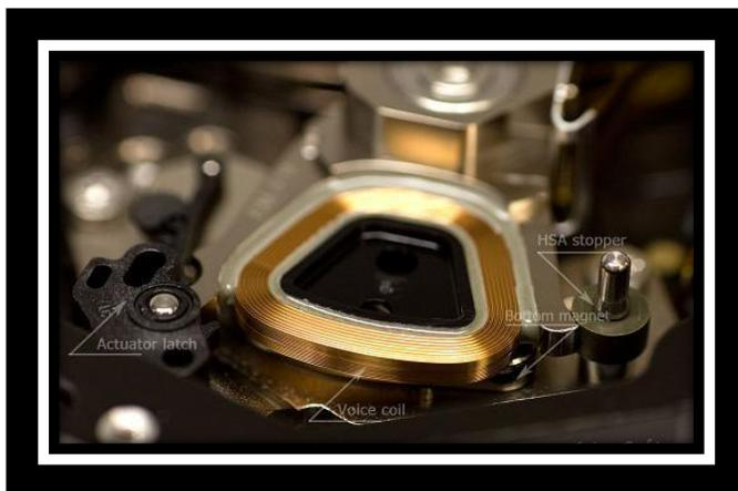
The Voice coil is a part of HAS and moves the head assembly. The actuator latch holds the heads in a parking position to prevent them slopping about when the drive is moved.
