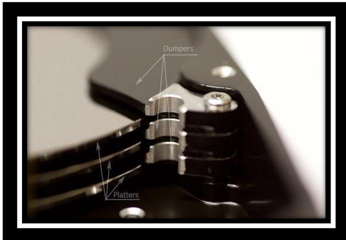
The Heads are mounted on the Head Stack Assembly and has a parking position.
