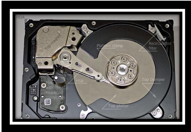
Data is stored on rotating disk platters. The platters are made of polished aluminium or glass and are covered with several layers of different compounds including ferromagnetic layer which actually stores all the data. Dampers or Separators located between platters reduce air fluctuations and acoustic noise.
