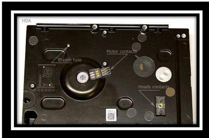
The spindle motor is shrunk into the casing and electrical supply is made via contacts that mate with the PCB. Shown is a breath hole that equalizes the air pressure within the HAD. This hole feeds air into a duct channel that holds an air filter to prevent particulates entering the unit and damaging the read write heads.
