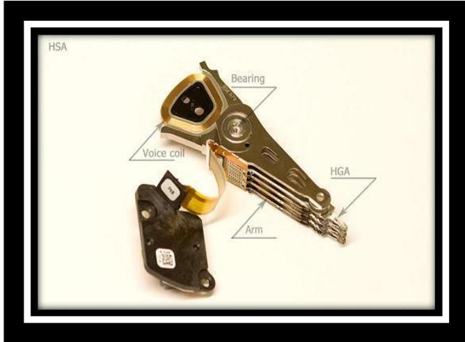
The HSA has a precision bearing with no play or movement. The connector to the PCB is airtight.
