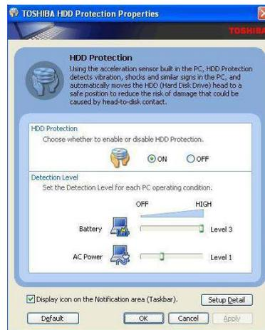
The protection level is temporally maximized 10 seconds after actions such as closing the LCD or unplugging the AC adaptor on the assumption that the notebook may be shortly picked up. The 3D sensitivity will also automatically go up as the tilt angle increases.
