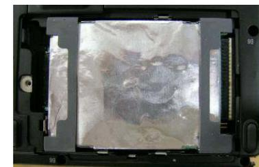
*Shock absorber material is added around the hard drive disk and works as a corner bumper mechanism*
